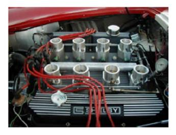
Figure 16 – View of Engine Converted to Run on Hydrogen
