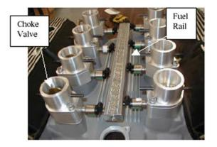
Figure 5 - Choke Assembly and Fuel Rail
