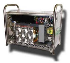
Close up of the 1 kW fuel cell used in the fuel cell ferry demonstration by DCHT. Provided courtesy of Enable Fuel Cells.
