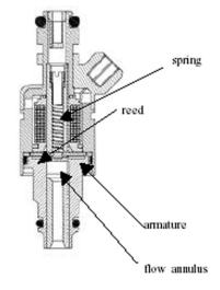
Figure 2 - Cross-section of injector
