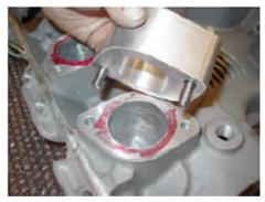
Figure 6- Match porting injector with intake manifold
