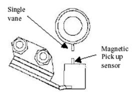
Figure 15 – View of Distributor with missing vane
