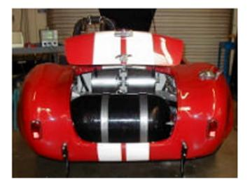
Figure 7 – Hydrogen storage tank
