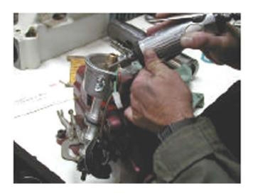
Figure 14 – Grinding out 7 of the 8 vanes.
